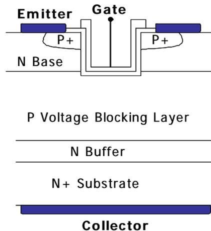
Figure 2: p-channel IGBT using conventional N+ Substrate.
